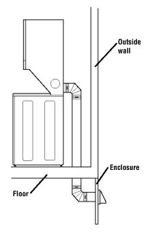
For mobile home use, gas laundry centers must be securely fastened to the floor. Order Mobile Home Installation Kit 346764 from your Sears store or Sears Service Center. Kit includes the necessary fastening hardware and detailed installation instructions. Exhaust system hardware is also available through your Sears store or Sears Service Center.
